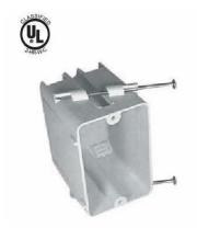
SINGLE GANG 23 Cubic Inch, Nail On Box 2-1/4" x 3-5/8" x 3-1/2" Four Knockouts Positioning tabs for Stud Mounting
